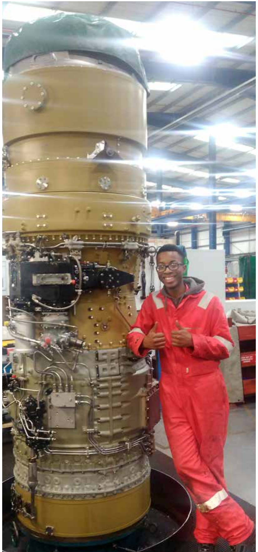
Devante is pictured next to an Industrial Avon Gas Turbine which is used to power an external turbine to either generate electricity, generate heat, or to pump oil & gas via pipelines either onshore or offshore. The engine is similar to an aircraft gas turbine but has been modified for industrial use.
