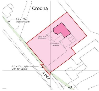
All vegetation within the visibility splay to be removed prior to construction of the site access.
