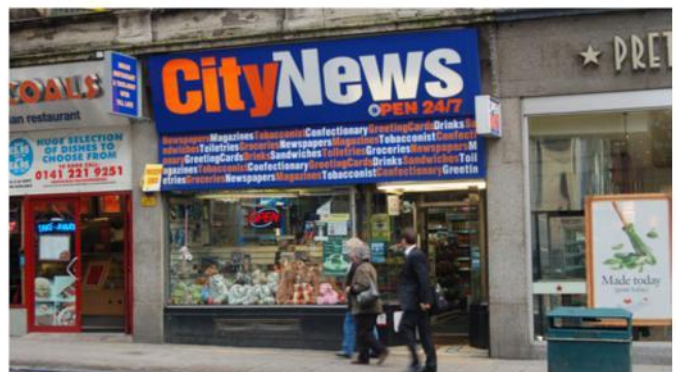
Fig 16 Poor signage which is back-lit, overly deep and blocking the clerestory. There are also excessive fixed and illuminated wall signs. ©Crown Copyright Historic Environment Scotland
